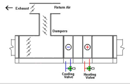
Dampers, heating and cooling valves for air handling unit.
